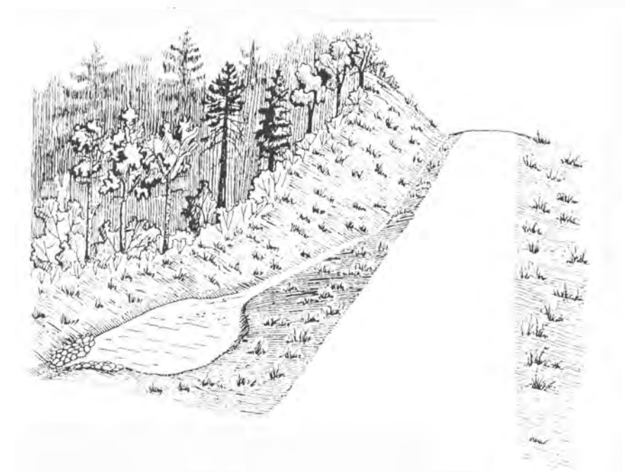
Figure 5-13 c. A sediment trap to slow runoff and trap sediment for channelized flow.
